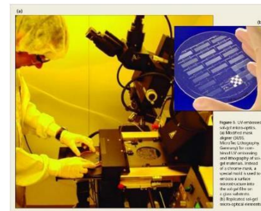
C2: Wafer Level Optics (WLO) on SUSS MicroTec Mask Aligner in 1997
